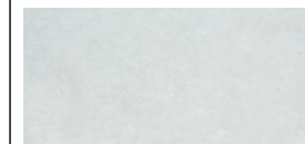
18 - Cemento bianco + finitura acrilica trasparente Natural white concrete + clear water repellent finish
